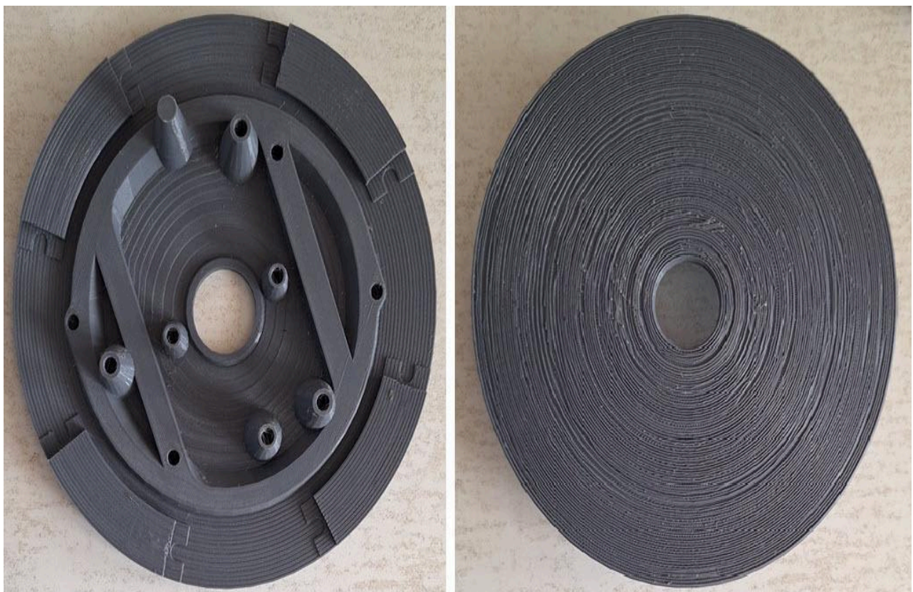
Figure 6: Initial 3D printed models of hybrid hot plate. Bottom view (left) and top view (right).
