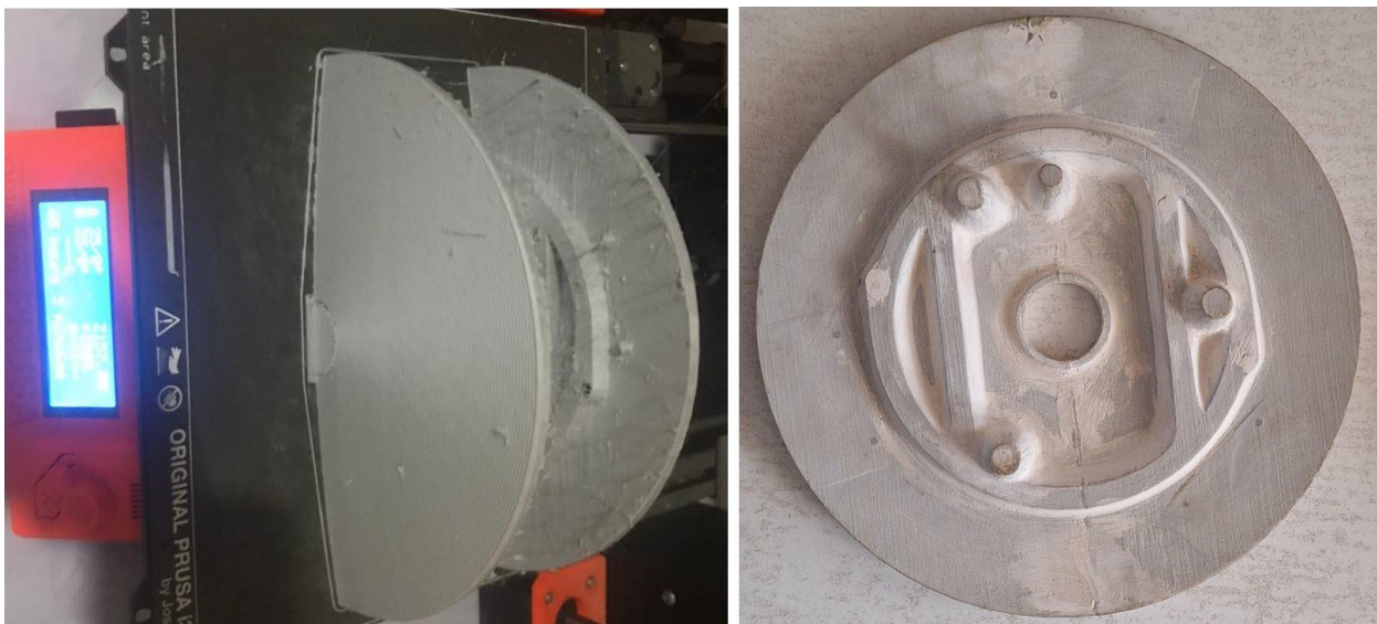
Figure 8: 3D printed model with a casting release agent to its surface.
