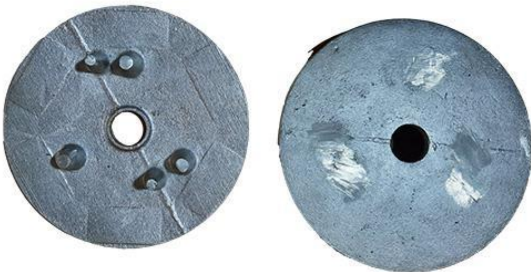
Figure 11: Aluminium casting for PTC-only hot plate before surface finishing
