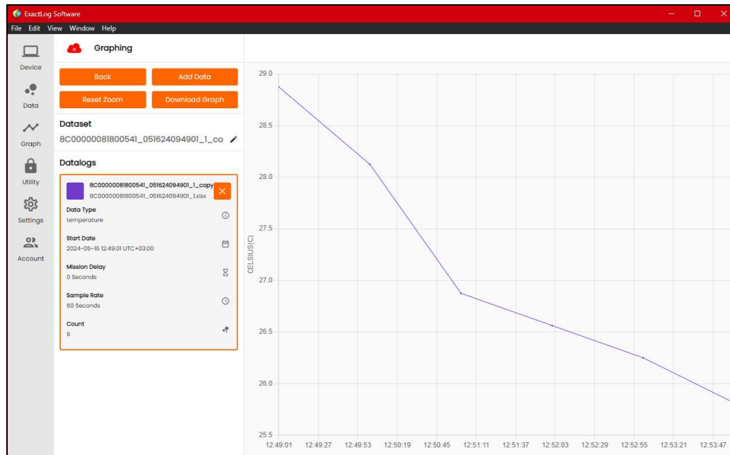
Figure 24: PC software for analysing the data collected from the thermochron sensor
