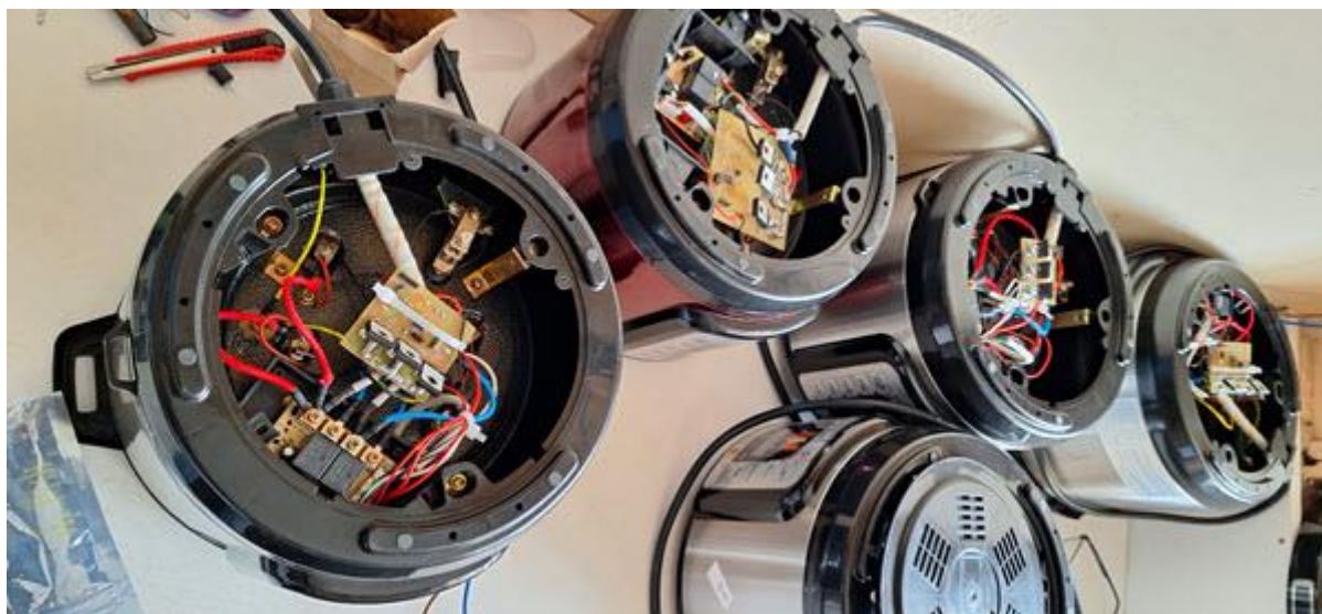
Figure 20: Modified DC EPCs ready for cooking tests
